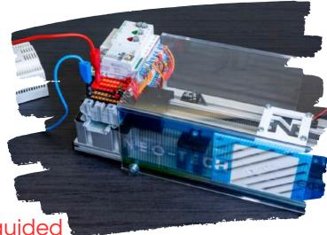
DC linear axis with belt-driven guided carriage with µ-controller or PLC drive
